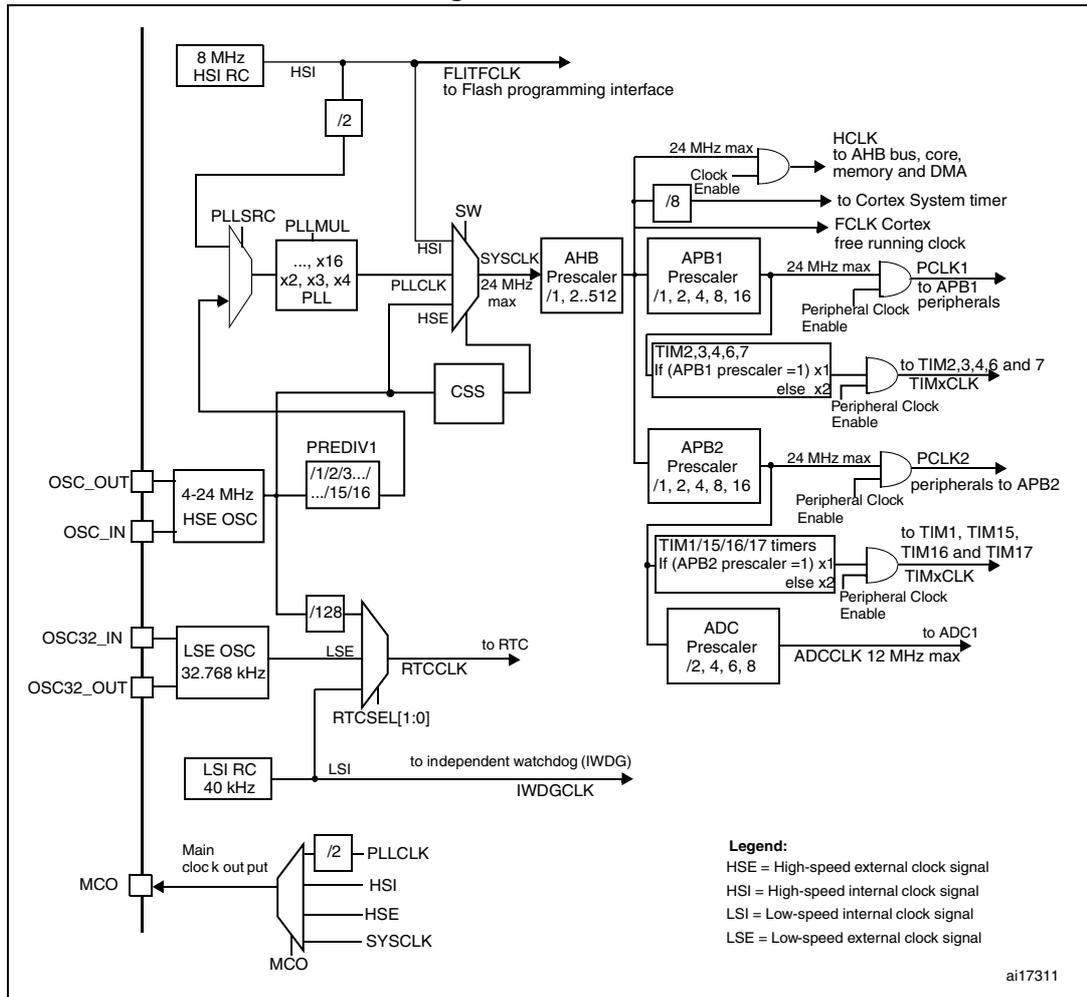
1. To have an ADC conversion time of 1.2 μs, APB2 must be at 24 MHz.
