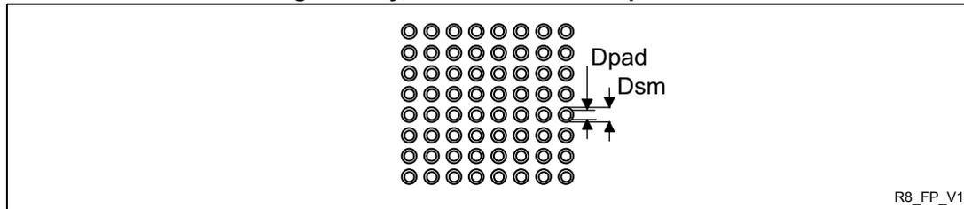
**Table 51. TFBGA64 recommended PCB design rules (0.5 mm pitch BGA)**
