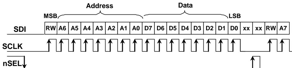
Figure 1. SPI Timing
