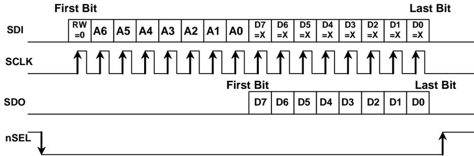
Figure 2. SPI Timing—READ Mode
