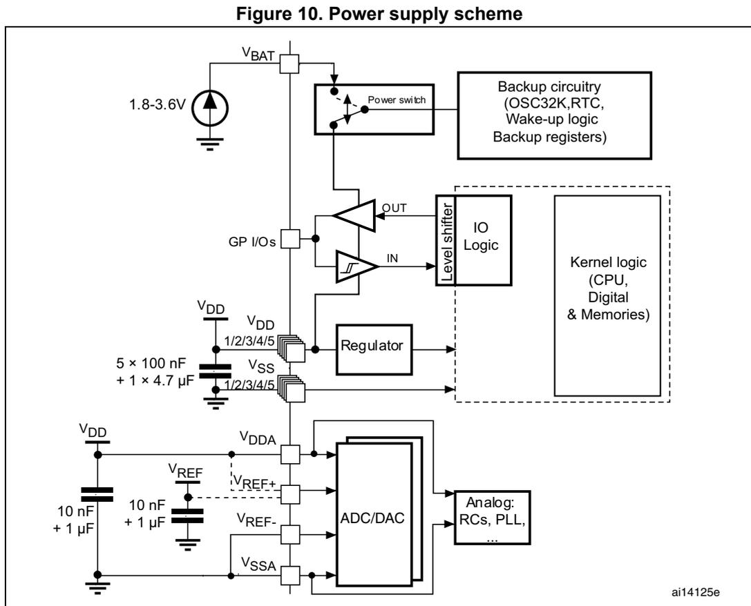
**Caution:** In [Figure 10](#), the 4.7 μF capacitor must be connected to V<sub>DD3</sub>.
