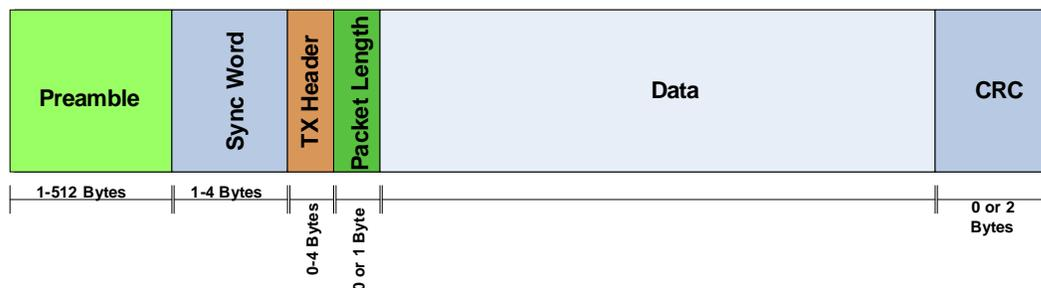
Figure 12. Packet Structure
