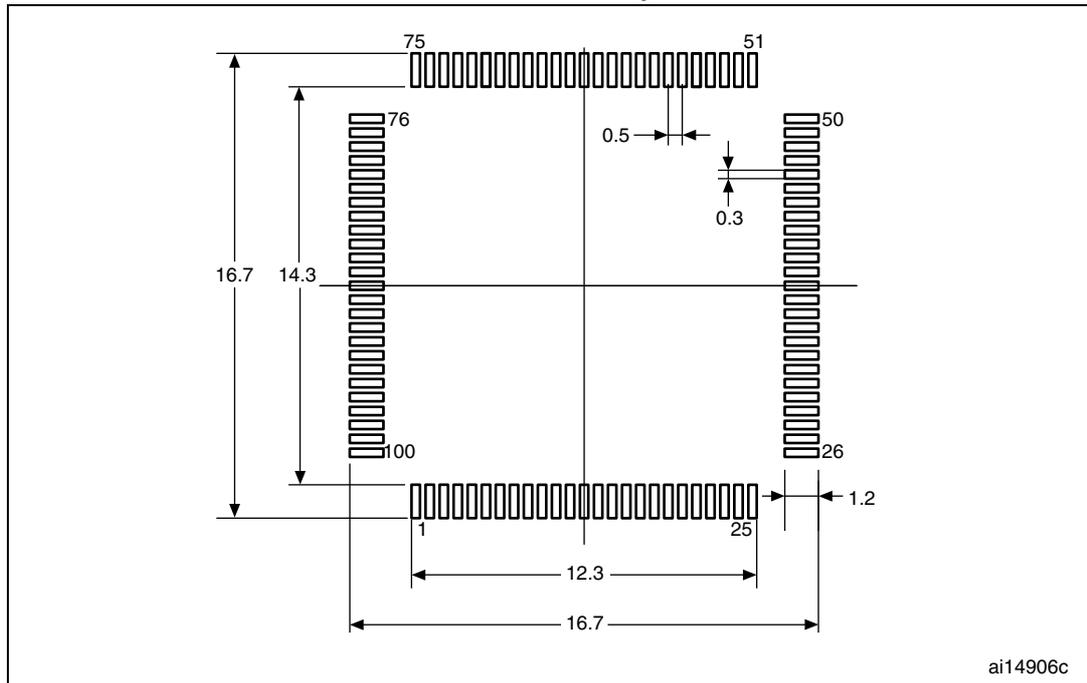
1. Dimensions are in millimeters.
