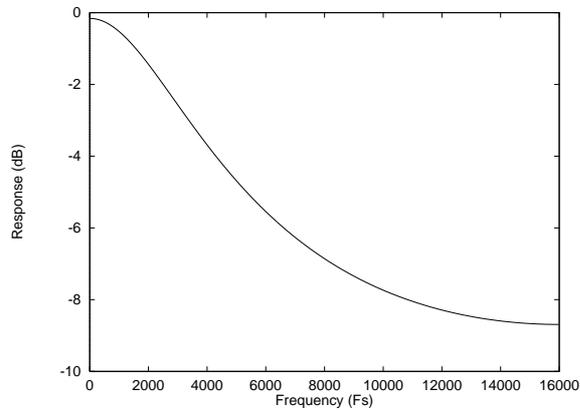
Figure 51 De-Emphasis Frequency Response (32kHz)
