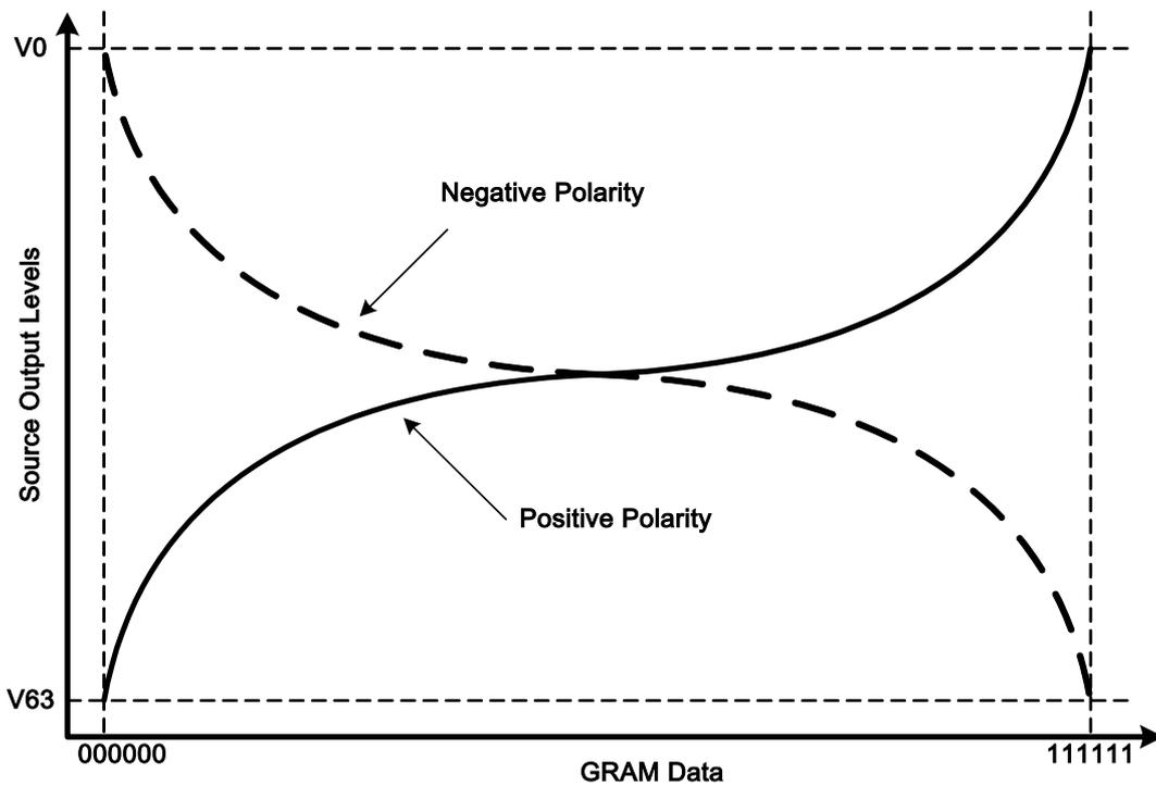
Figure 40 Relationship between GRAM Data and Output Level
