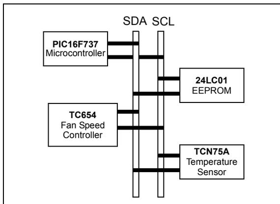
**FIGURE 6-2:** Multiple Devices on I<sup>2</sup>C™ Bus.
