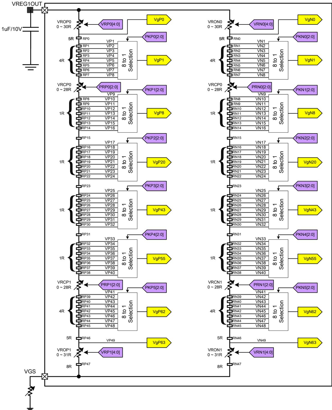
Figure 37 Grayscale Voltage Adjustment
