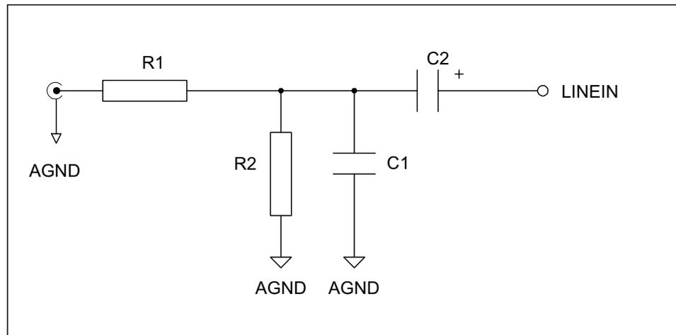
**Figure 11 Line Input Application Drawing**
