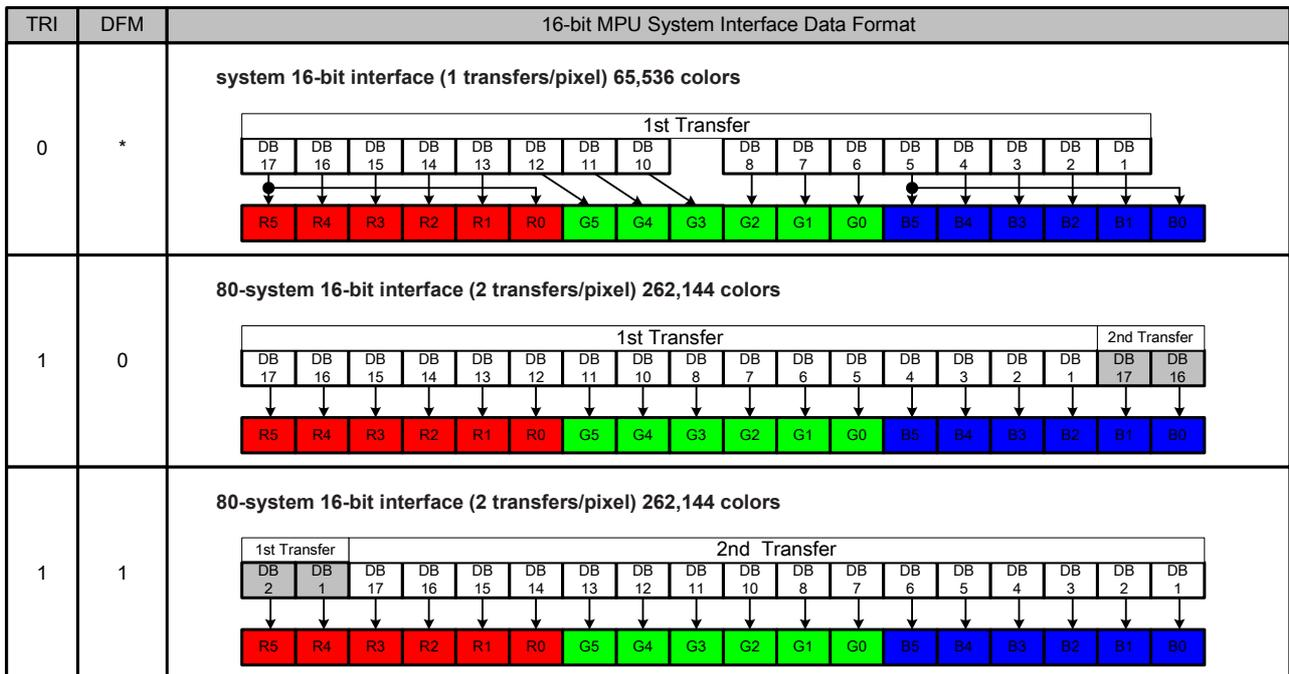
Figure26 16-bit MPU System Interface Data Format
