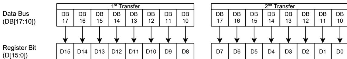
**Figure23 Register setting with i80 System Interface**
