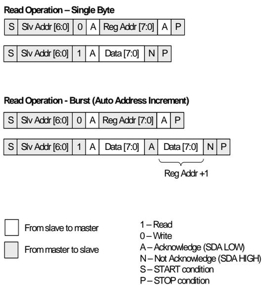
**Figure 10. I<sup>2</sup>C Read Operation**
