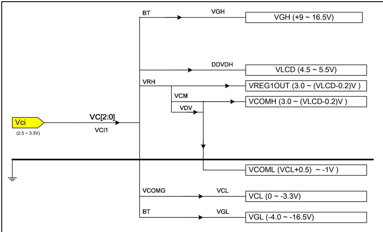
**Figure 45 Voltage Configuration Diagram**
