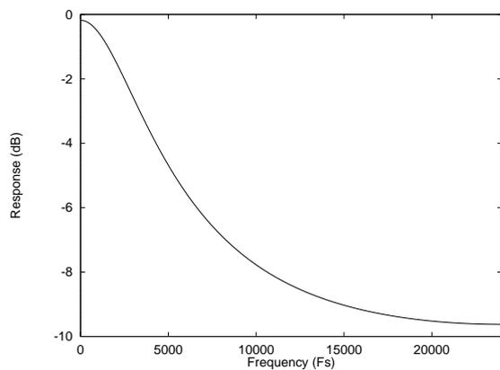
Figure 55 De-Emphasis Frequency Response (48kHz)
