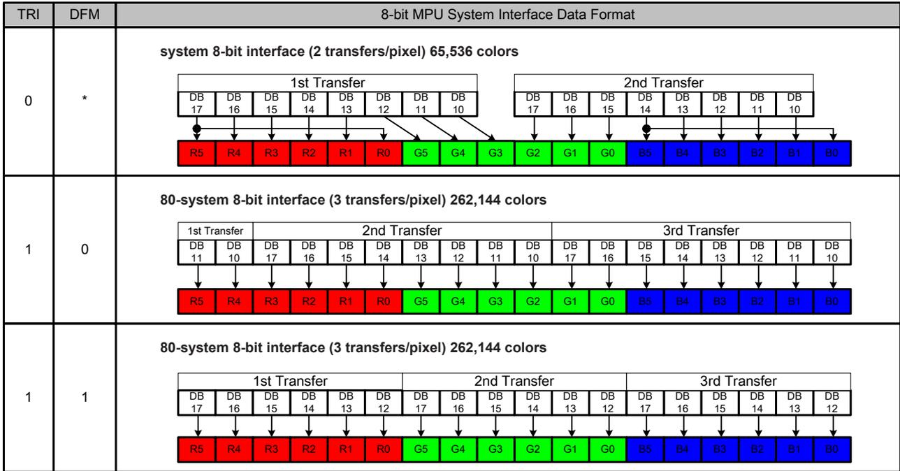
Figure5 8-bit System Interface Data Format
