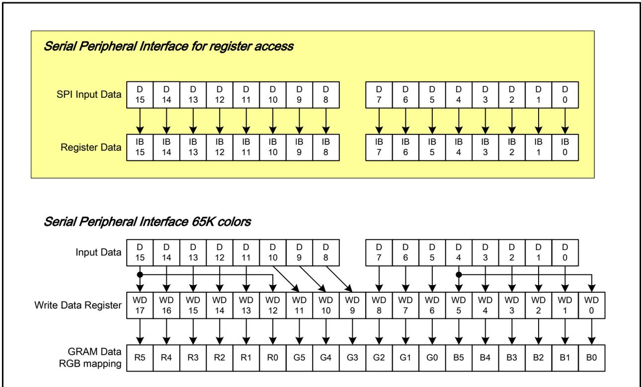
**Figure 7 Data Format of SPI Interface**
