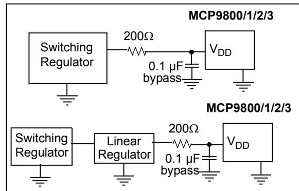
**FIGURE 6-3:** Power-supply Filter Using a Single Resistor.
