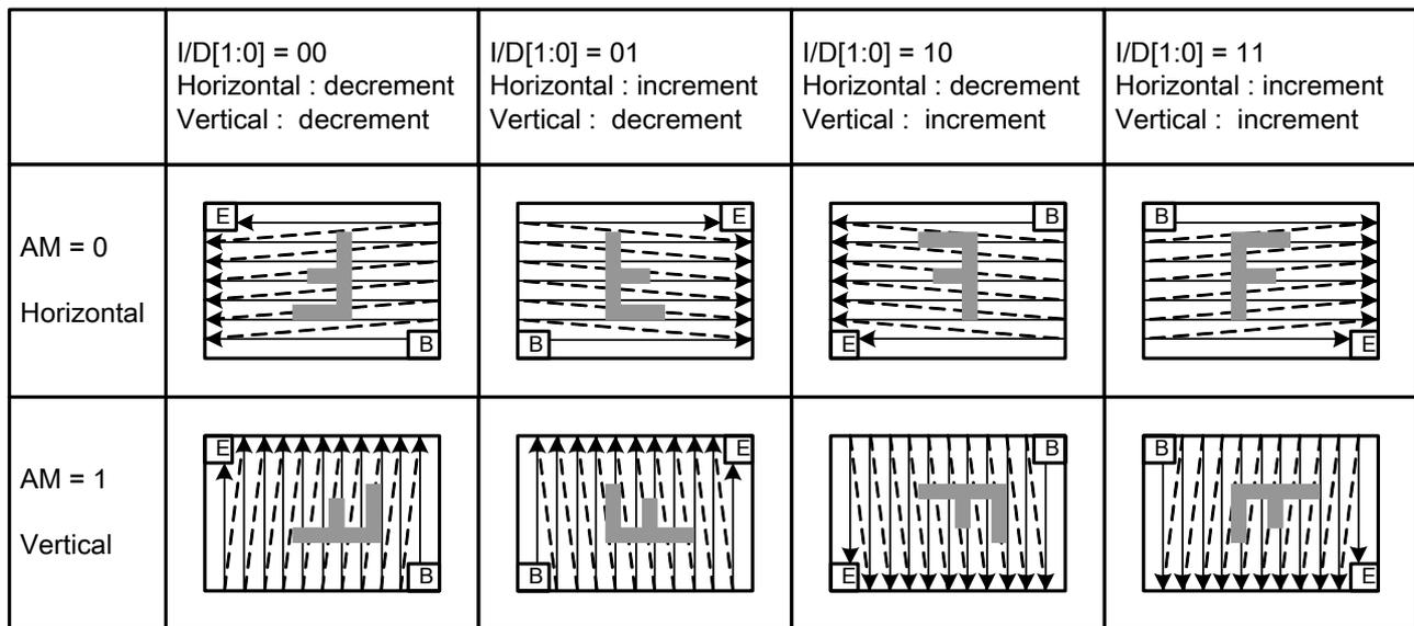
**Figure25 GRAM Access Direction Setting**
