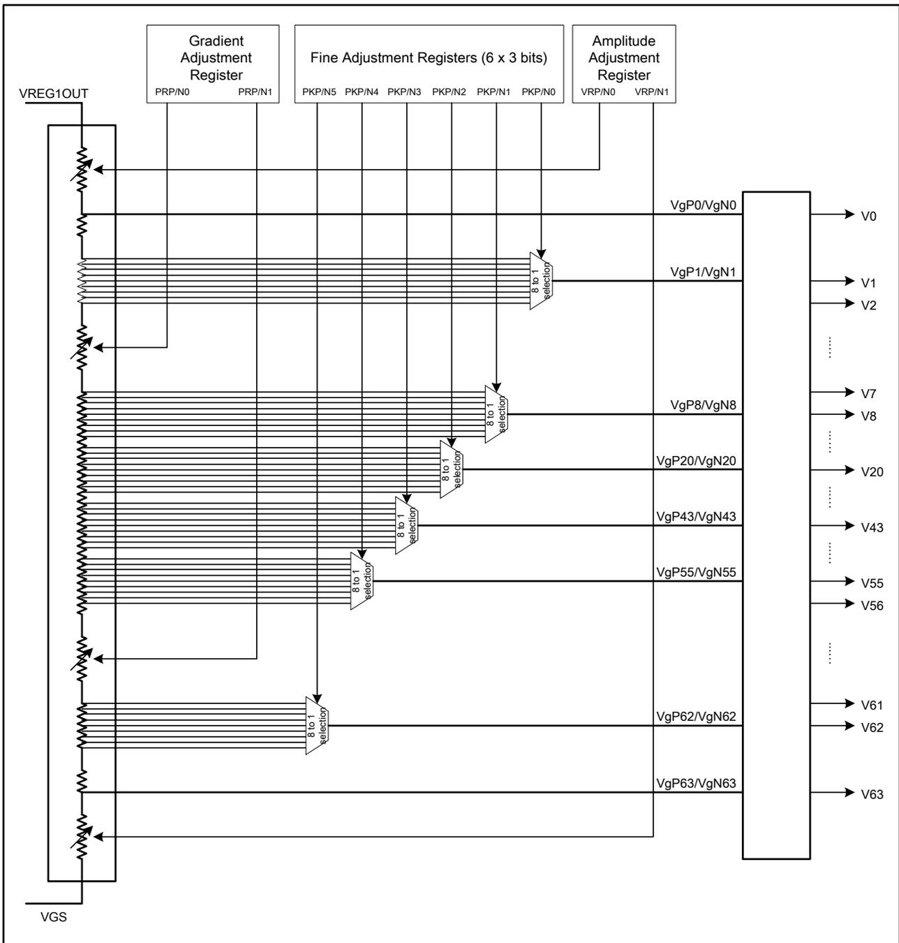
**Figure 36 Grayscale Voltage Generation**
