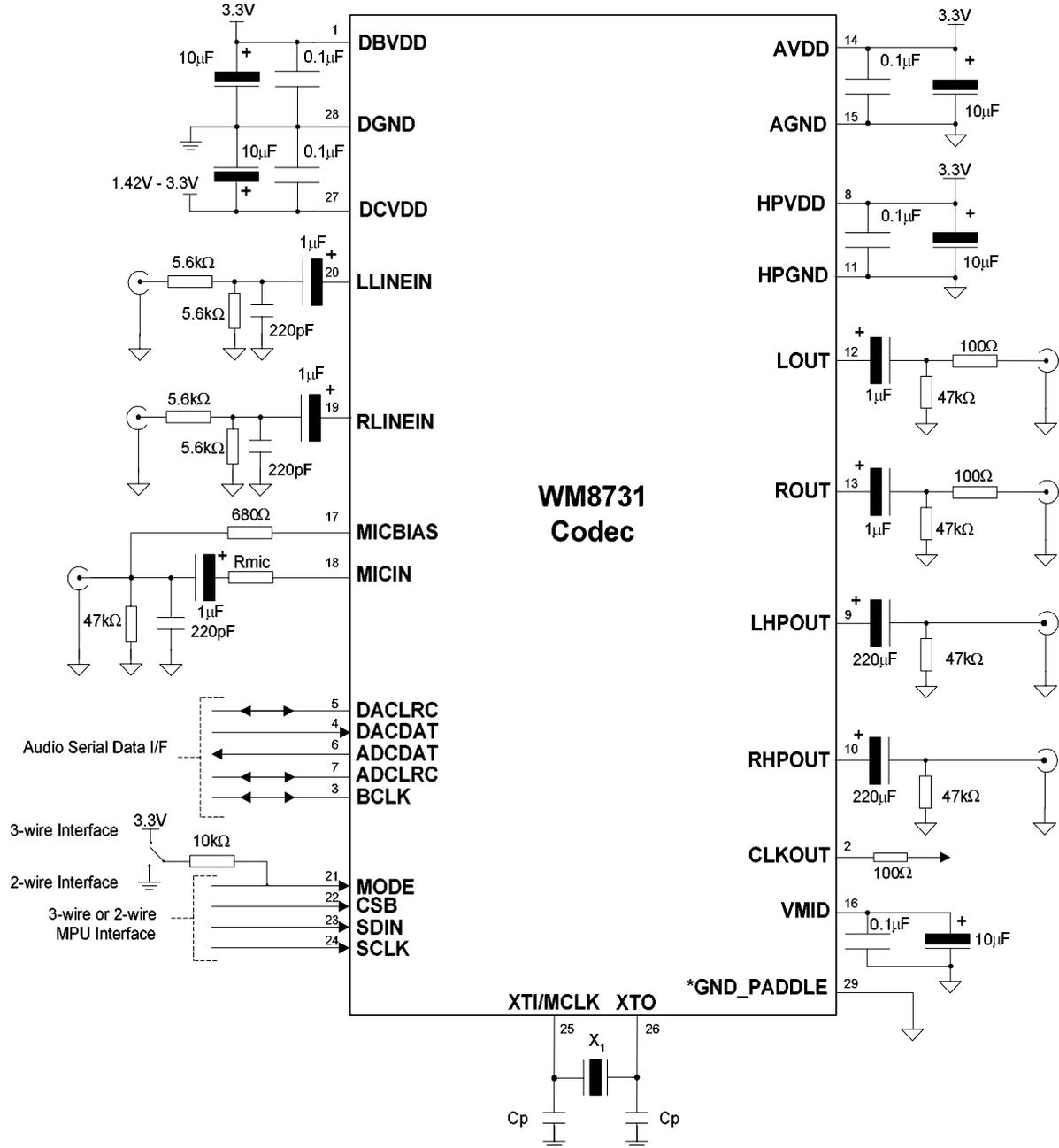
Figure 57 External Components Diagram
