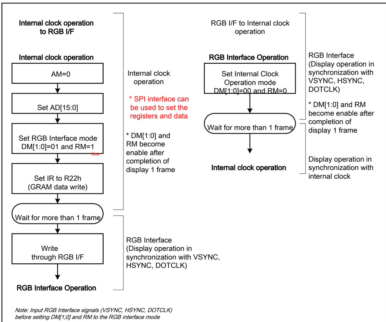
**Figure19 Internal clock operation/RGB interface mode switching**
