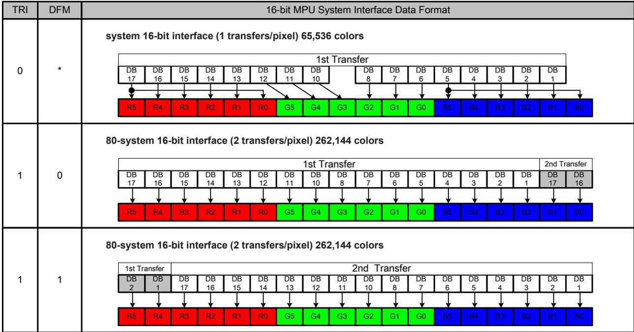
**Figure3 16-bit System Interface Data Format**
