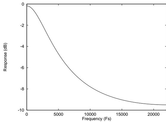
Figure 53 De-Emphasis Frequency Response (44.1kHz)
