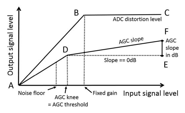
**Figure 1:** Relationship between input and output signal level WITH  $(A \rightarrow D \rightarrow F)$  and WITHOUT  $(A \rightarrow B \rightarrow C)$  an automatic gain control (AGC) with an indication of some of the WDSP AGC parameters that can be controlled by the user. Inspired by a paper by Phil Harman: "A discussion on the AGC requirements of the SDR1000" (I added the relevant AGC parameters for better understanding).
